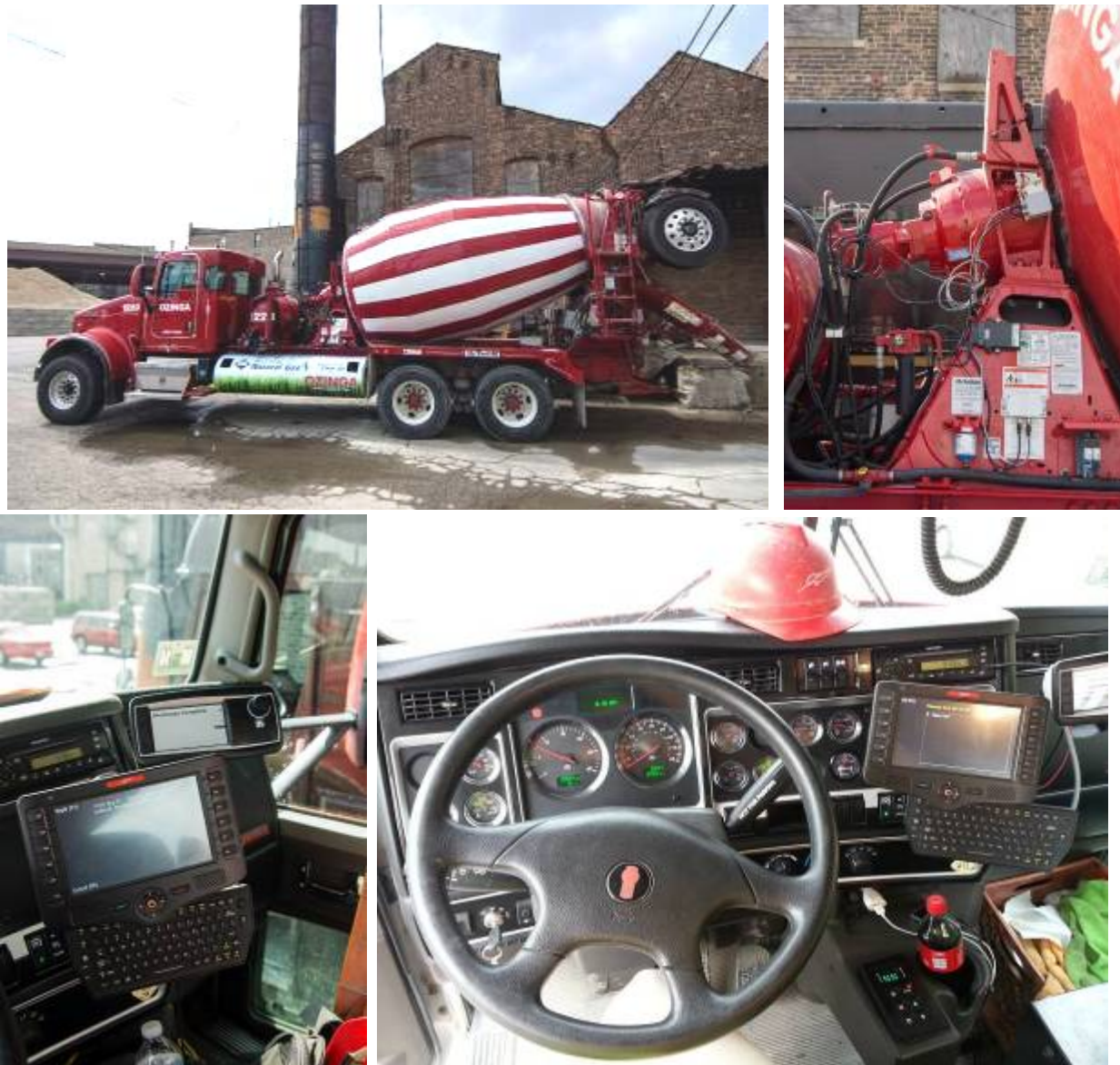
Figure 7- Truck mixer equipped with the VERIFI system
