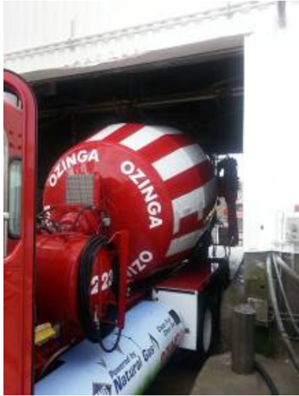
Loading concrete into truck mixer at batching plant
