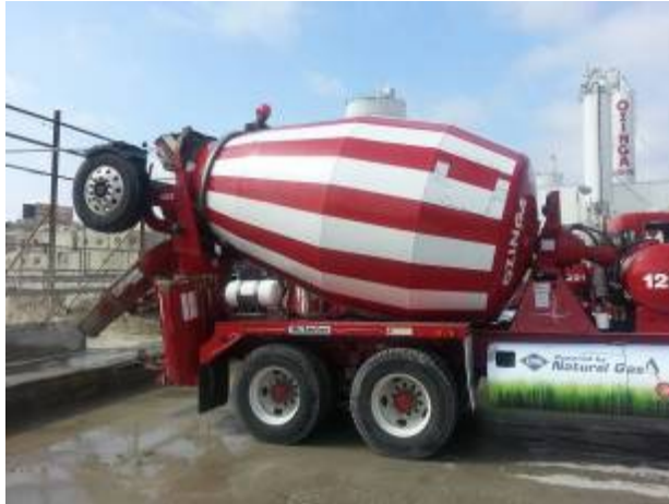
Initial mixing at batching plant
