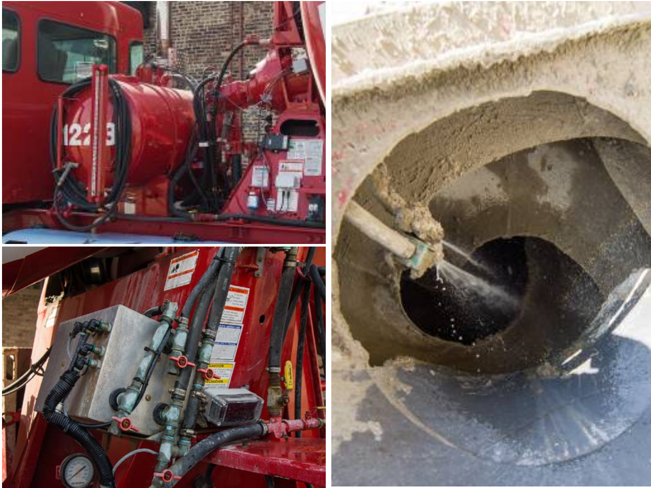
Figure 27- VERIFI water addition and flow meter system
