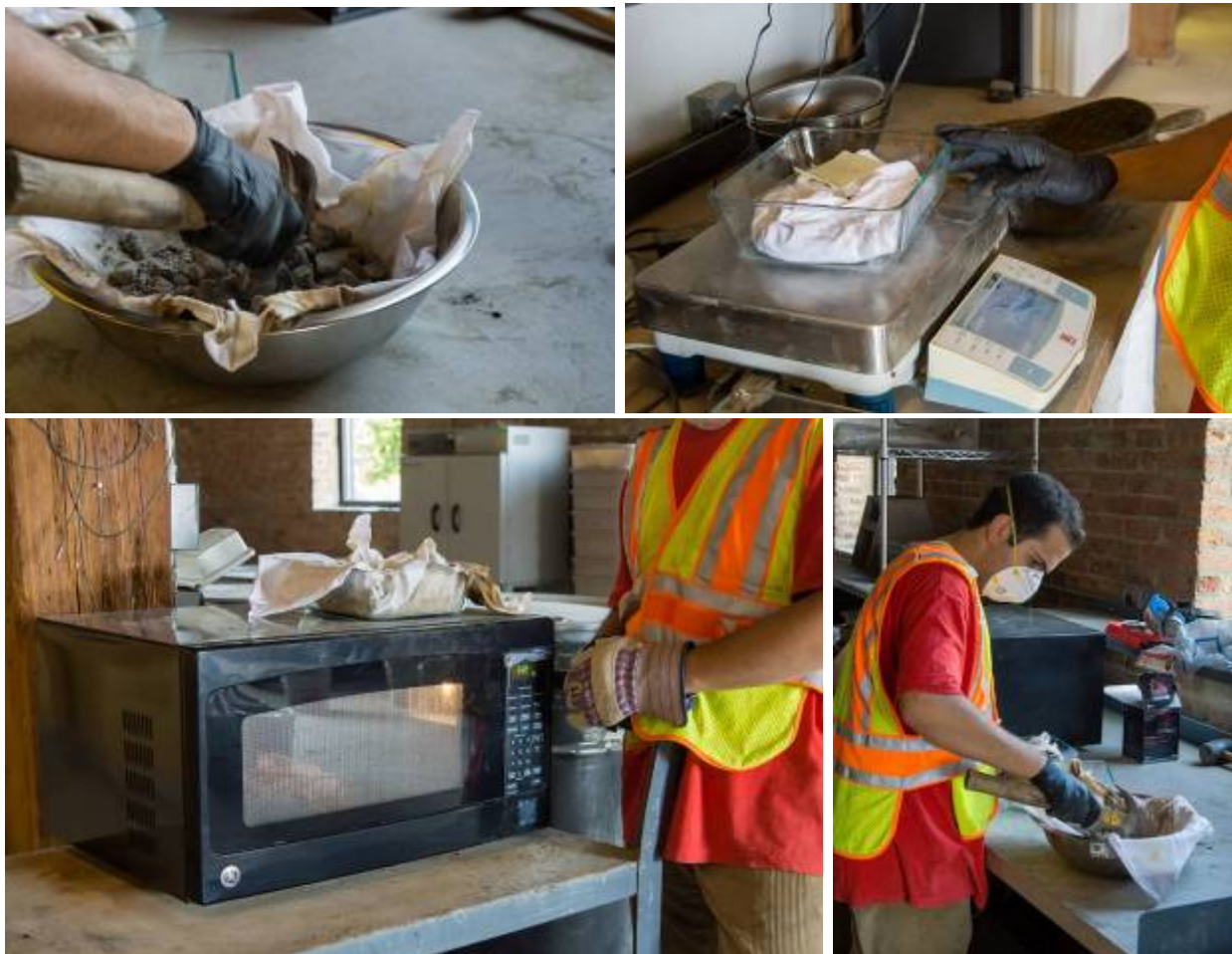
Figure 12- Test of water content of freshly mixed concrete using microwave oven test
