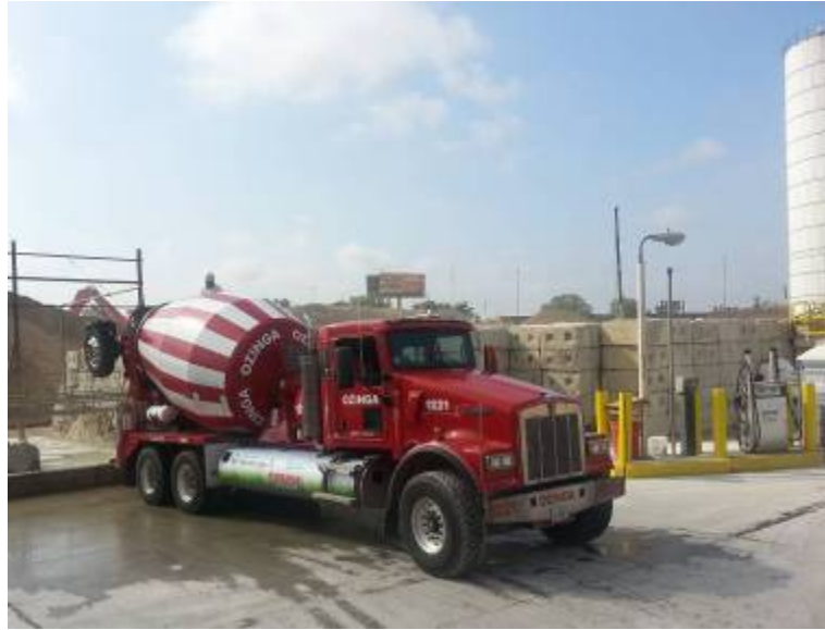
initial mixing before leaving batching plant
